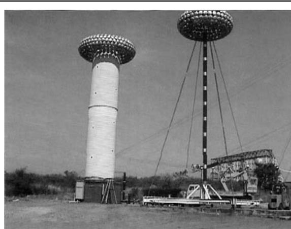
*Fig.1: A view of 5000kV/500 kJ outdoor impulse voltage generator with damped capacitive divider*
